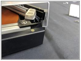
• To remove the cover, lift it straight up on all three corners. You will then need to gently pull out on the silver sides (one corner at a time) to un-hook the cover.
