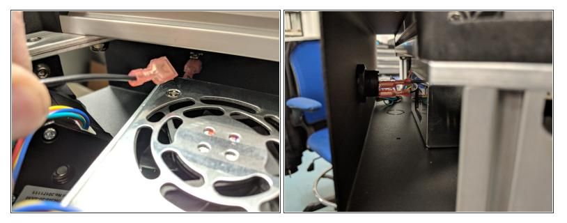
The power switch connector (black wire with spade crimp, exiting the Z tower wire bundle)
