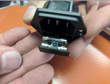
Open the fuse drawer on the IEC connector. Insert the two fuses that were provided into the location. as seen in the image. Close the drawer.
